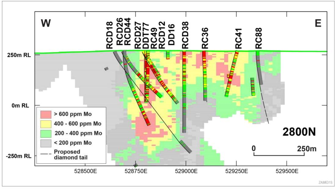
Drill cross-sections (west-east) through the Anthony deposit show high grade zones surrounded by lower grade mineralisation. Drill holes have intersected potentially ore-grade molybdenum mineralisation down to 500m depth below surface. The deposit shape is conducive to a large open-pit mining operation 贯穿安东尼矿体钻探横截面(东西方向)显示了高品位区被较低品位矿体环绕。钻孔穿过可计矿石品位的钼矿矿体至地表以下500米。矿藏形状有利于大型露天开采
