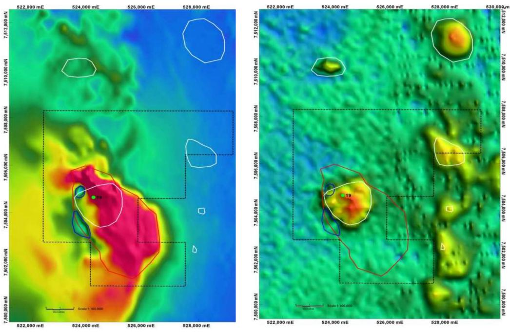
The target is an untested magnetic anomaly with a coincident potassium anomaly indicating an intrusive igneous complex. There has been no previous detailed exploration 该靶区是未经勘测的磁异常及钾异常重合,隐射出侵入类型火成岩综合体。该处之前从未进行过详尽的勘探工作
