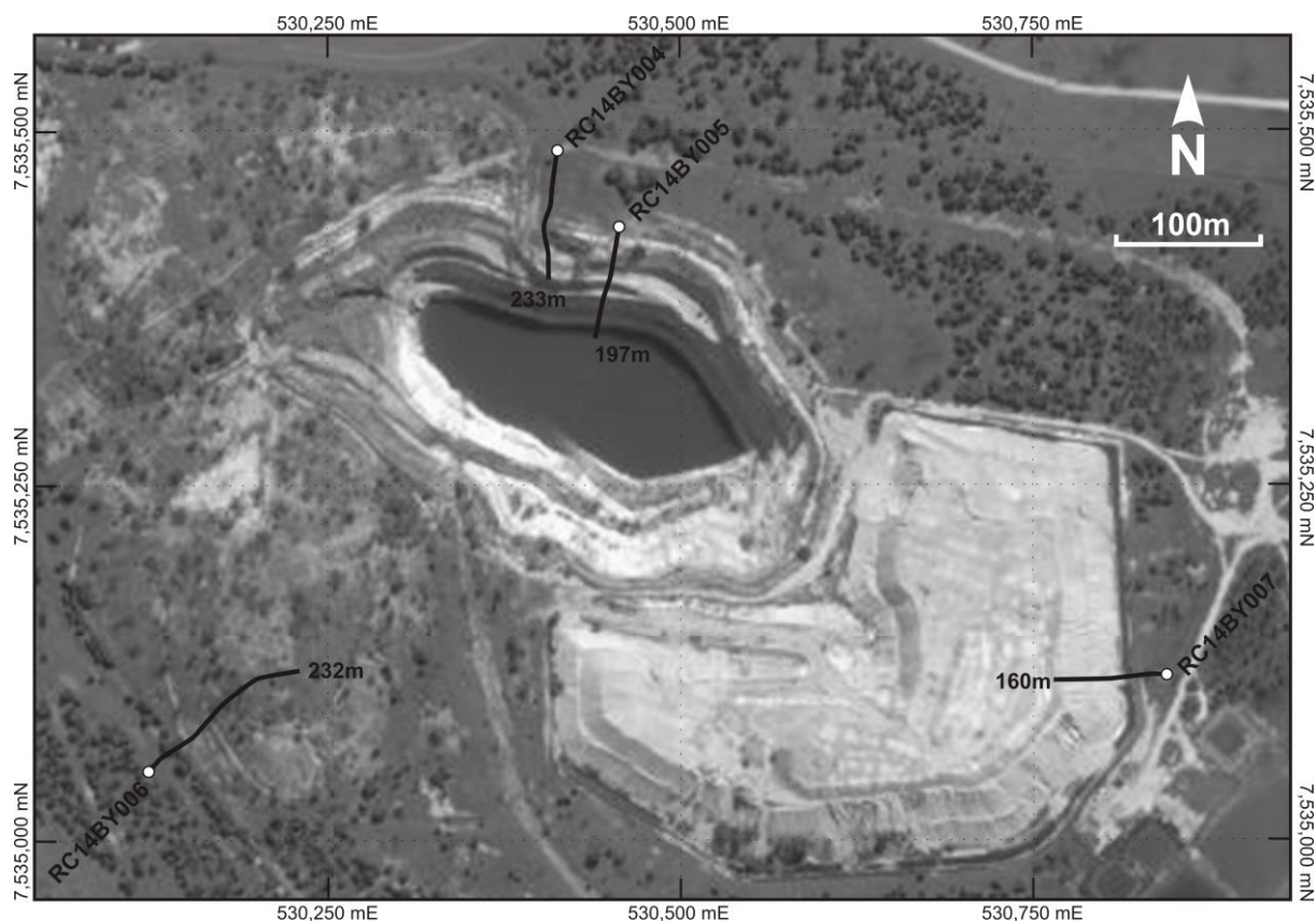
Figure 8: November 2014 drill holes shown on a satellite image of the the Belyando Gold Mine. Coordinates given are MGA 94, zone 55S.
