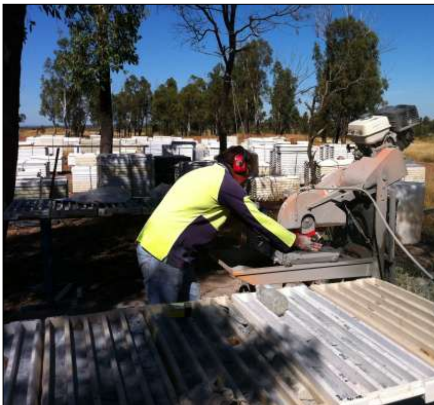
Diamond Drill Core being cut by a diamond saw at the Anthony project area
