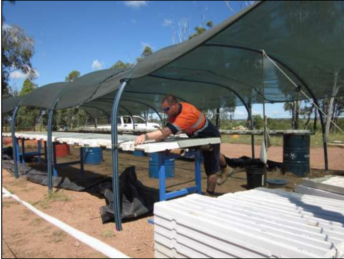
Figure 5. Detailed geological logging of Anthony diamond core
