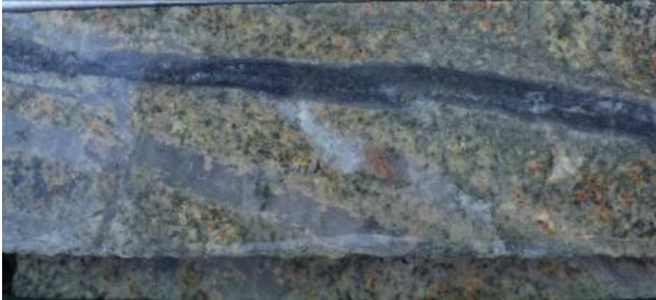
Detail of drill core showing quartz-molybdenite veins in brecciated & altered porphyry
