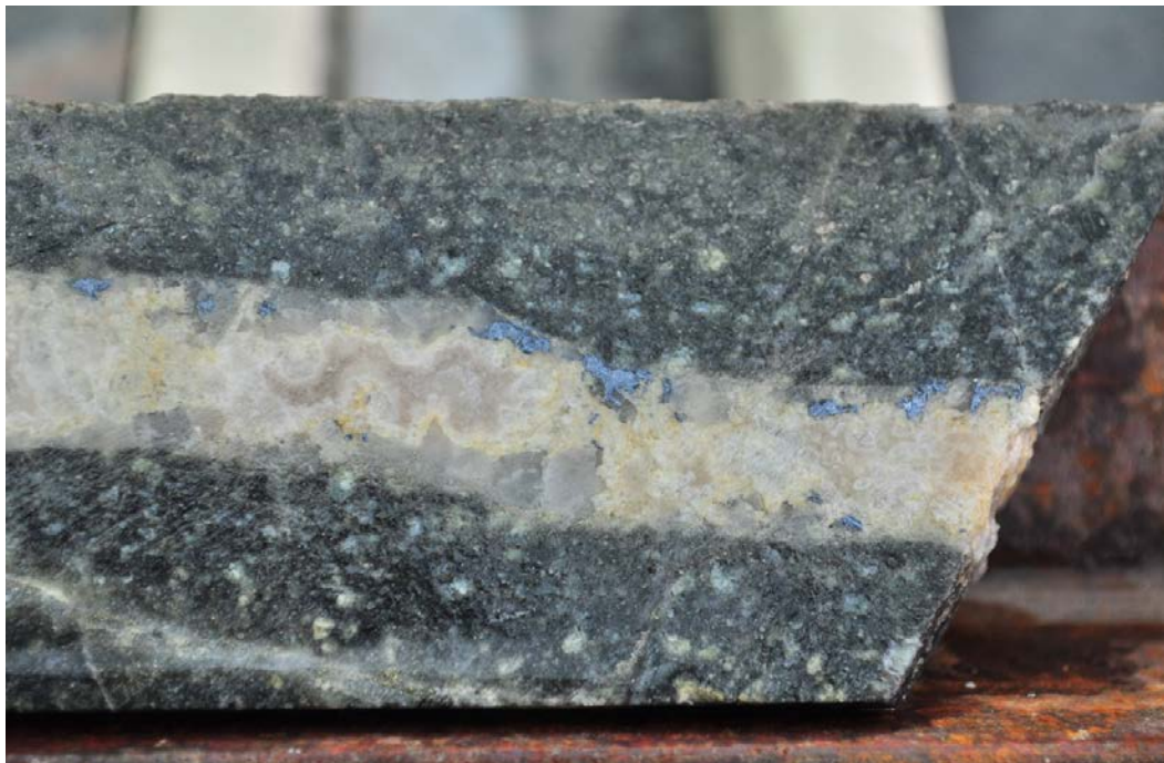
Anthony molybdenum deposit. Diamond drill core showing stockwork quartz-molybdenite veins within altered monzonite
