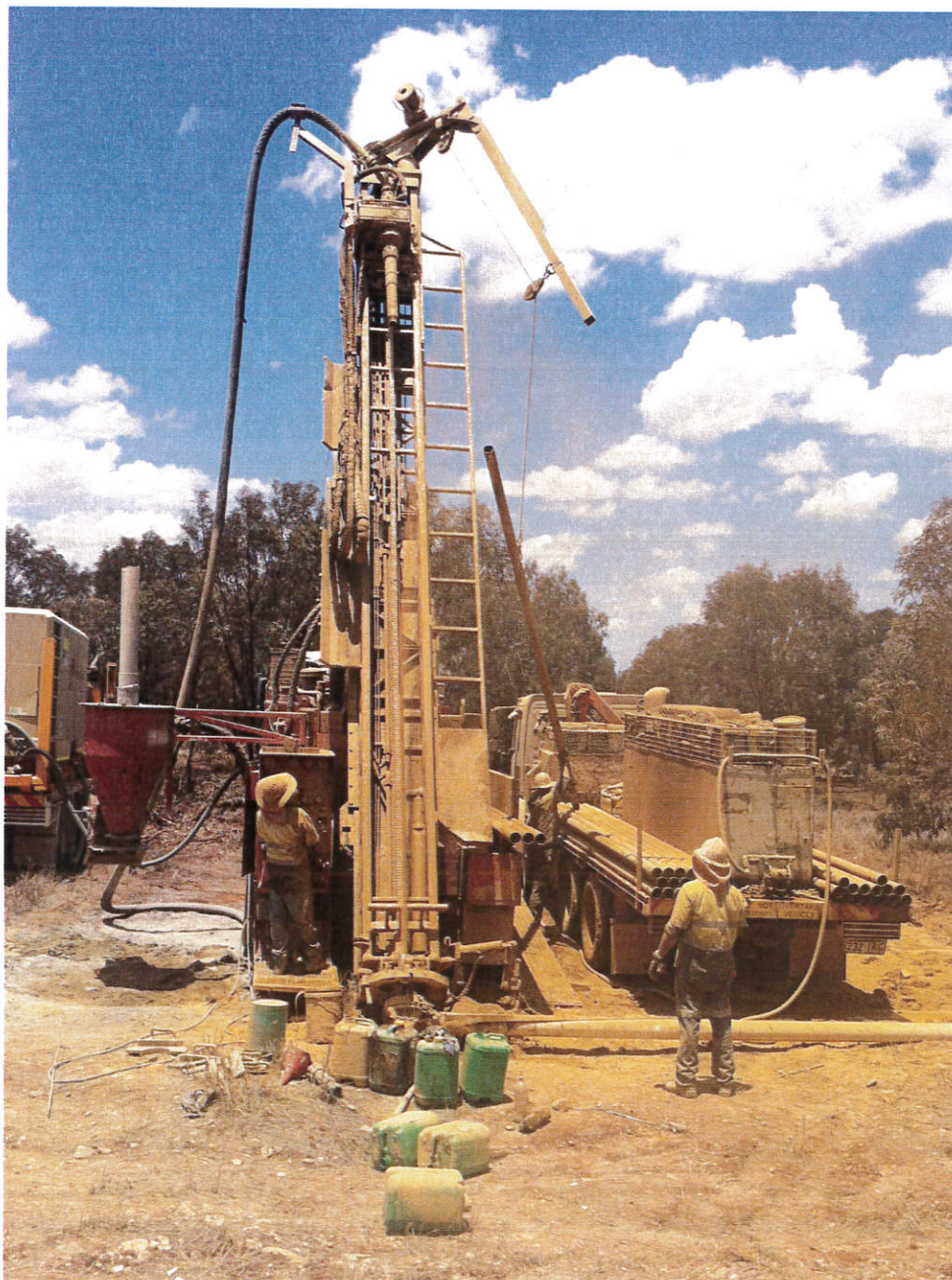
Drillers pulling rods after completing a drill hole at the Belyando Gold Project in November 2014
