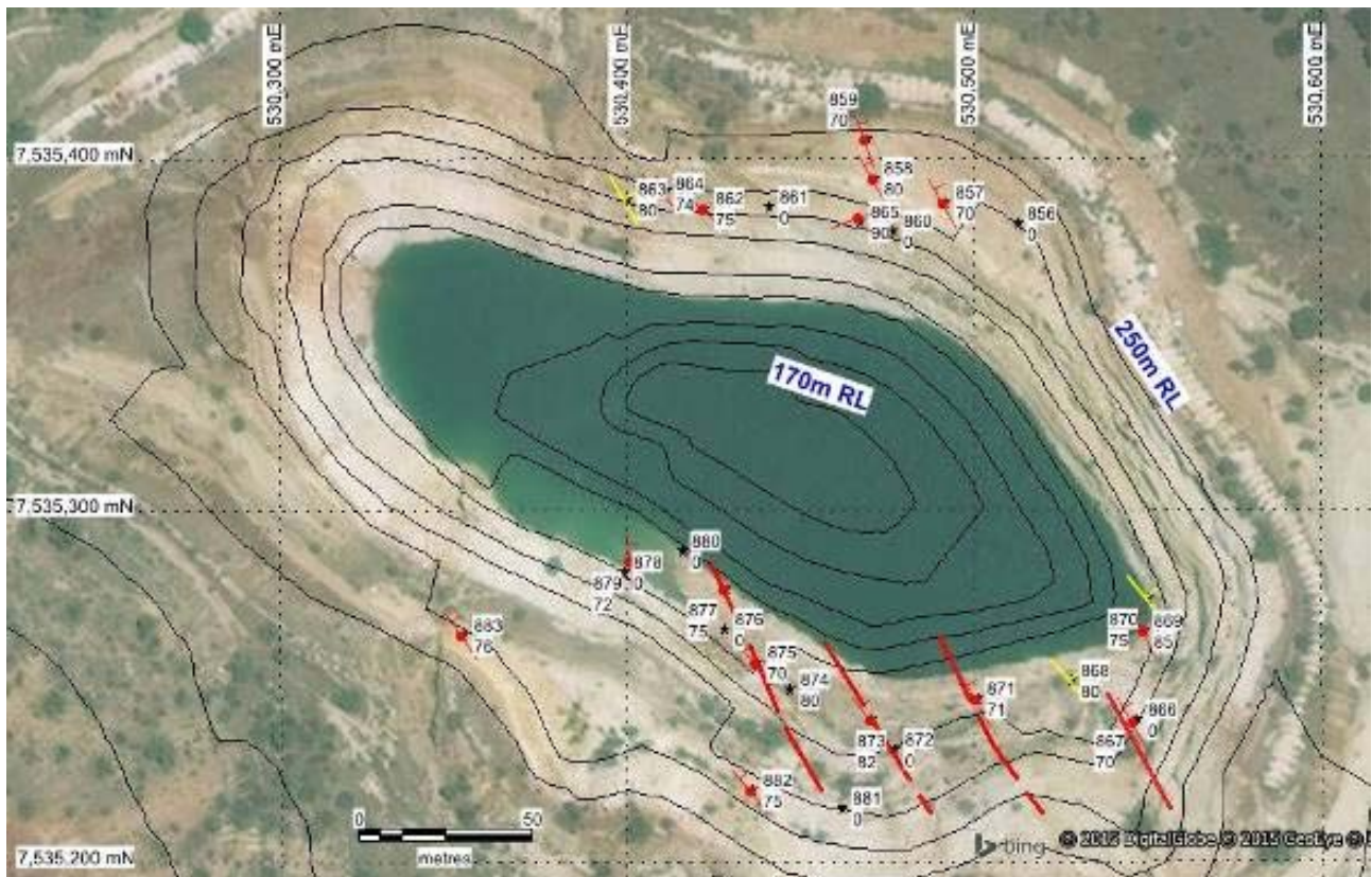
Figure 2. Quartz-pyrite lodes (red) mapped out in the accessible part of the Belyando pit, shown in aerial photography (CMC, 2015). Coordinates given are MGA94, Zone 55 south.
