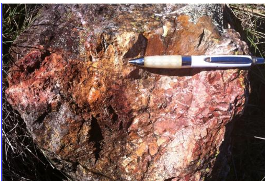
Hydrothermally altered silicified quartz-veined siltstone float from the Ti-Tree Ridge gold prospect
