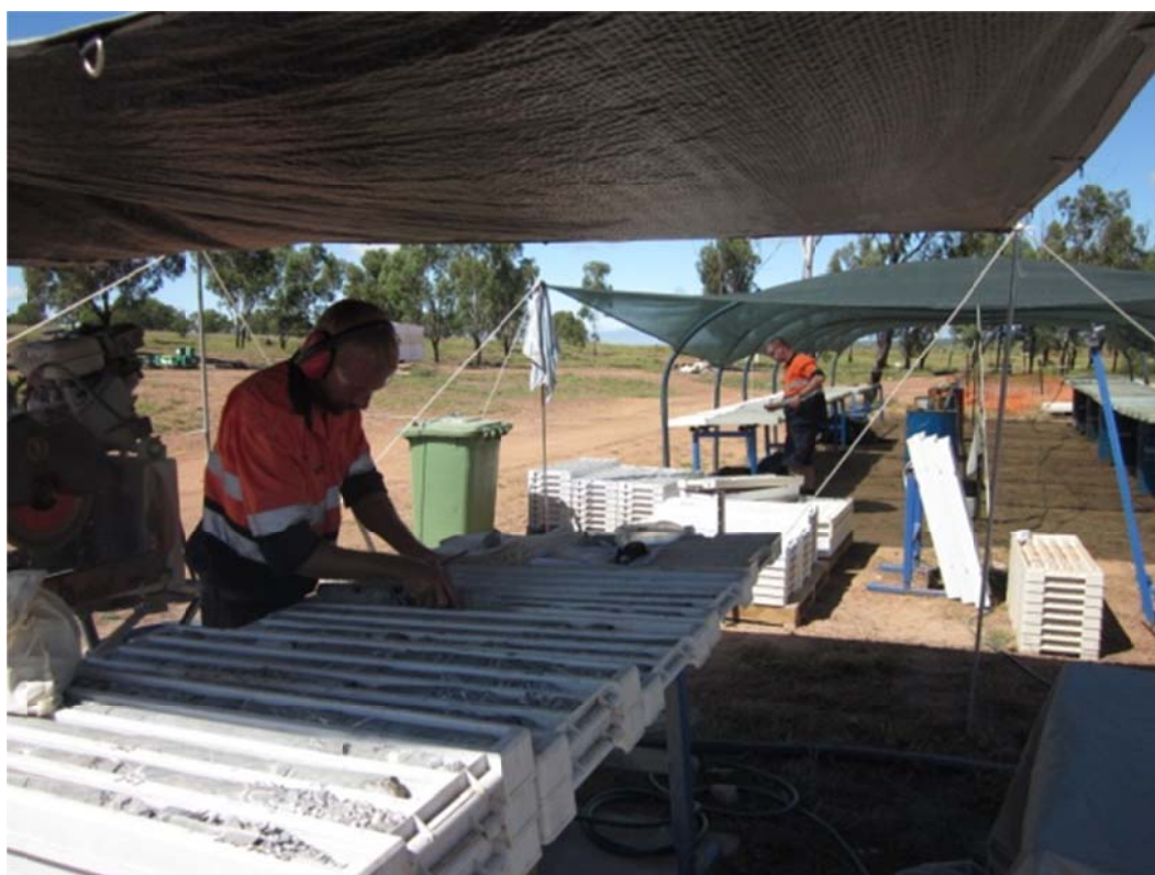
Figure 2. Anthony diamond drill core sampling
